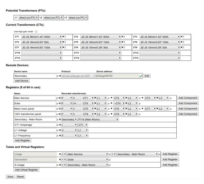
Figure 1: Example of eGauge Installation-Settings Page
