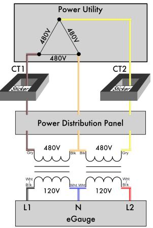
Transformers: 2x Functional Devices TR50VA008 480V/120V 50VA
