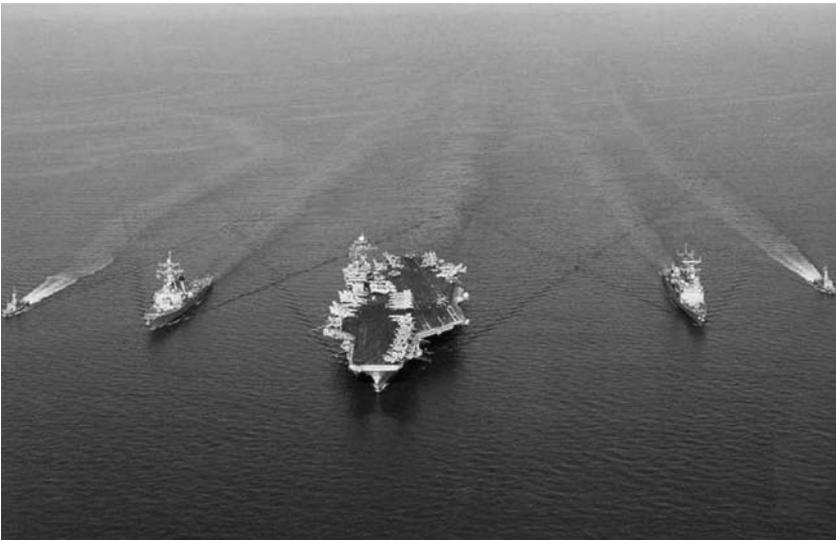
Figure 7.6 Large-scale Kelvin wakes. (Image source: US Navy).
