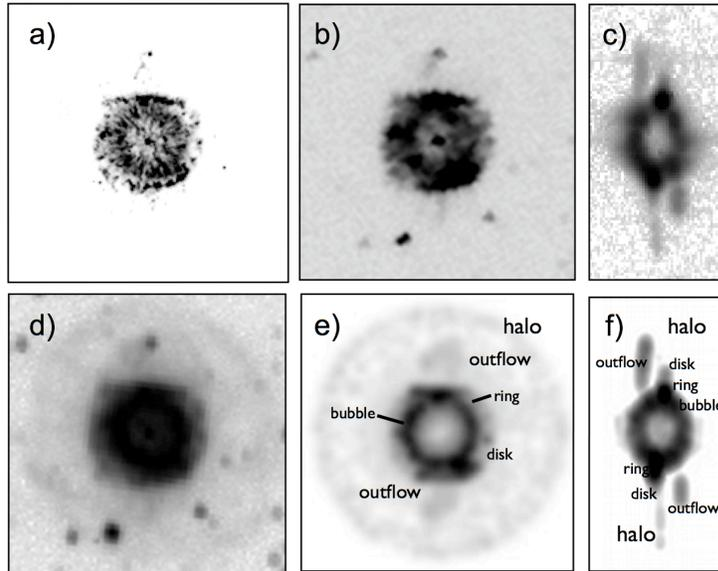
Figure 1. Here we compare various observational views of NGC 6751 with our Shape model. a) *HST* image, b) SPM,  $H\alpha+[N\ II]$  image, c)  $[N\ II]$  spectra for slit g, d) SPM  $[O\ III]$  image, e) Shape model, f) model PV diagram.
