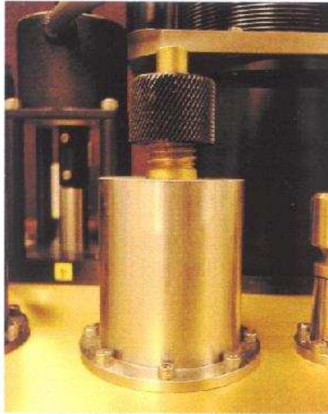
Figure 7-3: Fill Port Plug for LN 2 Precooler
