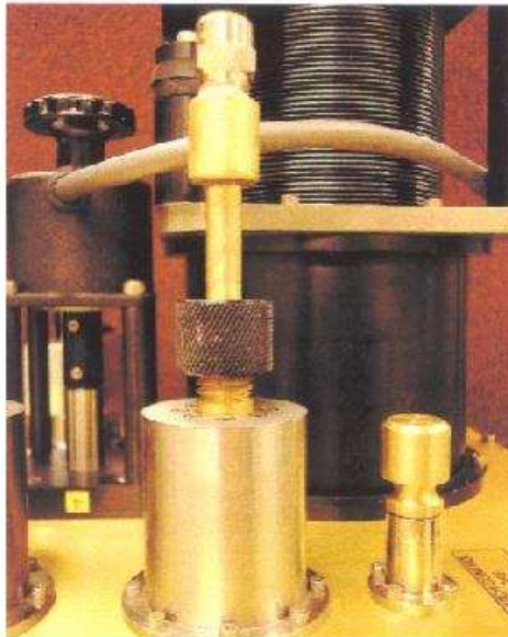
Figure 7-4: Pressure Relief Valve for LN 2 Precooler
