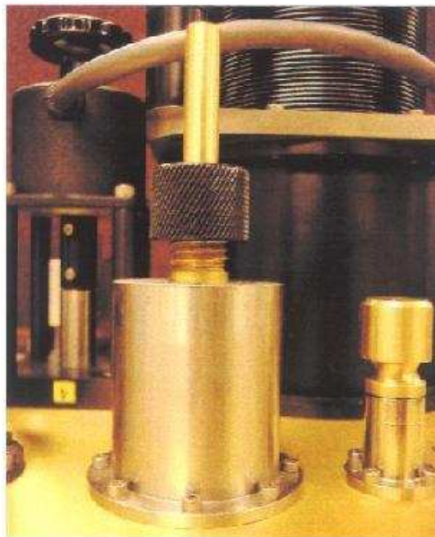
Figure 7-2: Fill Tube Extension for LN 2 Precooler
