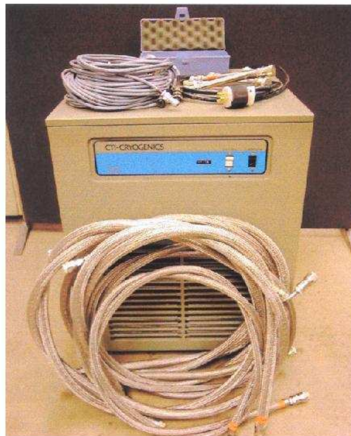
Figure 8-1: CTI Helium Compressor with Lines
